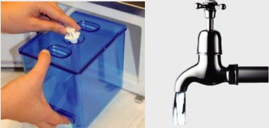
Fill blue cleaning container with cold water and connect it back to milk line.
