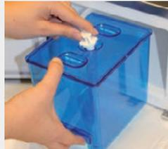
Un-plug milk line from blue container and plug back into milk container. Careful warm water inside blue container.
